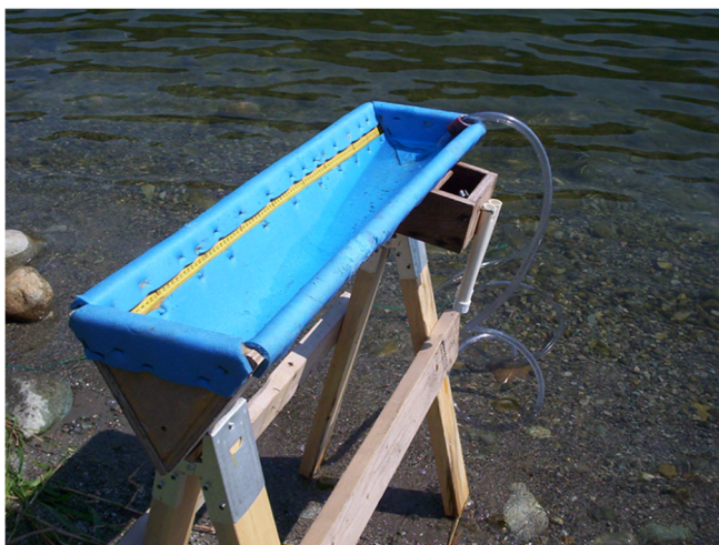
FIGURE 2 Water-filled padded fish sampling trough. The head of the fish is placed at the end with water inflow from a pump to ensure that oxygen levels remain high throughout the sampling event. A measuring tape has been integrated into the trough to simplify processing (Photo credit: Steven Cooke)
